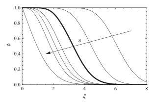
FIG. 2. Self-similar profiles  $\phi(\xi)$  for different values of n. Results of the numerical solution of Eqs. (14) and (15) for  $n = 1.25, 1.5, 2, 3, 4, 6, \infty$ . The thick line is the graph of the function given by Eq. (20) overlaying the profile for n = 2.
