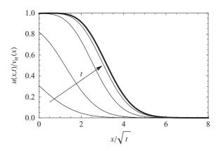
FIG. 1. Example of the collapse of the solutions of Eq. (7) onto a universal master curve at large times. Results of the numerical solution of Eq. (7) with n = 2 and  $\alpha = 1$ . Thin lines show snapshots of the solutions corresponding to t = 0.1, 1, 10, 100 (the direction of time increase is indicated by the arrow). The bold line shows the asymptotic master curve.
