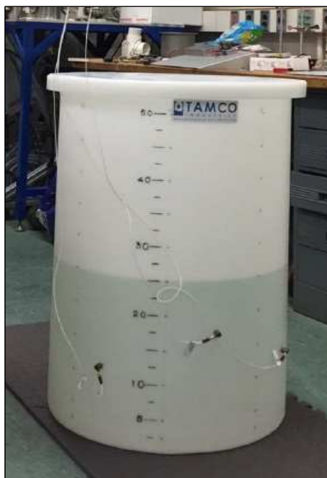
Figure 10. The 200-liter tank used in liquid modes counting tests.
