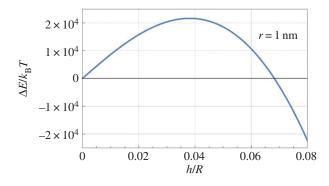
**Figure 2.** The dependence of  $\Delta E(r, h)$  on *h* for r = 1 nm in the case of a spherical water drop at 20°C with radius  $R = 10 \ \mu m$  charged to  $Q = \frac{1}{2}Q_R$ . (Online version in colour.)
