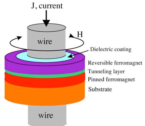
Fig. 1. Schematics of the proposed design.
