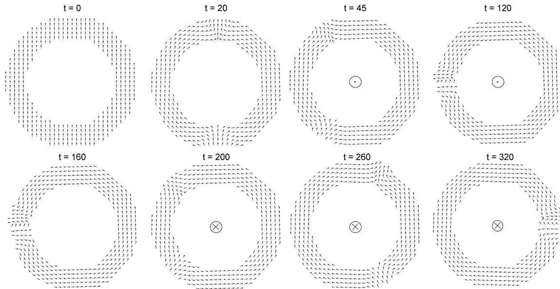
Fig. 3. Dynamics of the magnetization reversal in a ferromagnetic nanoring subject to the magnetic field from a wire passing through the ring center. Results of the numerical simulations of (3) (see text for details).
