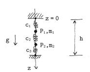
Consider the system shown in the figure, composed of two heavy points,  $P_1$  of mass  $m_1$ , and  $P_2$  of mass  $m_2$ , free to slide along a vertical guide and connected by three ideal springs with a rest length of 0, as in the drawing.
