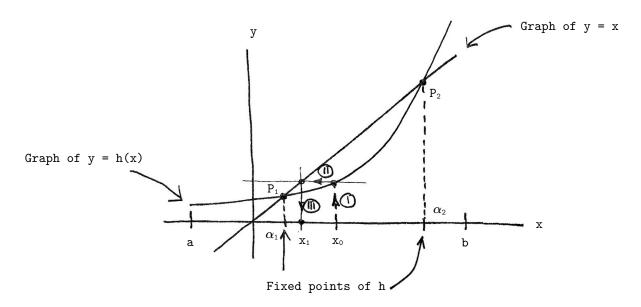
Represent on the same Cartesian plane the portions of the graph of the function y = h(x) which defines the one-point method to be examined and of the straight line graph of the function y = x, on an interval [a,b].
