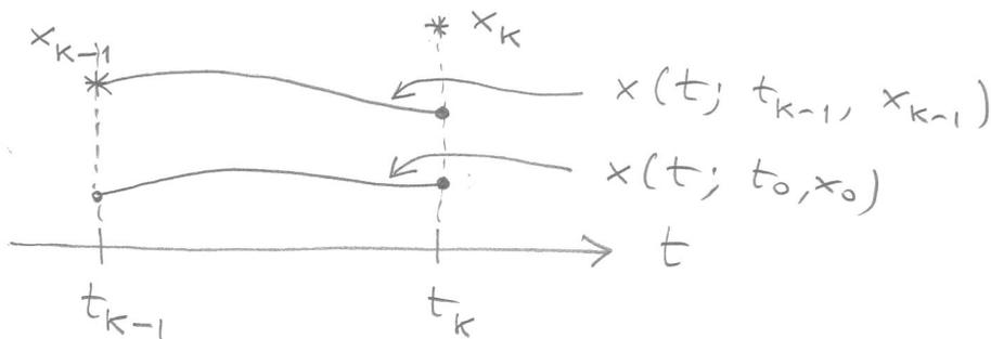
$$et_k = el_k + \varphi(et_{k-1}) = x(t_k; t_{k-1}, x_{k-1}) - x(t_k; t_0, x_0)$$
