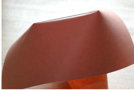
Fig. 8. A real sheet of paper undergoing a single fold. The ideal folding line is drawn to put in evidence the stretching
