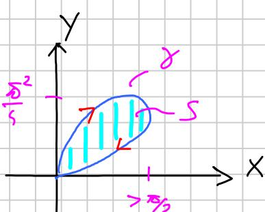
$$(L) \text{ GAUSS-GREEN } \vec{E} = (x, 0) \rightarrow \text{AREA} = \int_{\partial S} x \, dy$$
